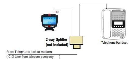
IMPORTANT: If using the parallel setup, you will still need to plug in a telephone handset to the PHONE socket (at least temporarily) to program your call blocker.
