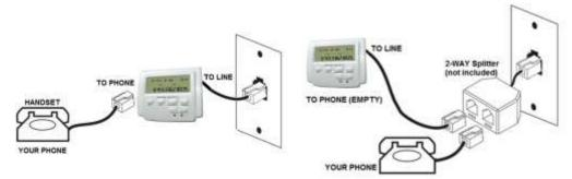
Important: If using the parallel installation option above, you will need to connect a telephone handset to the PHONE socket (at least temporarily) in order to do any programming or change any settings.
